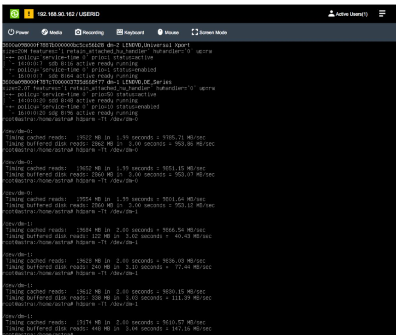
The screenshot shows a terminal window with the IP address 192.168.90.162 / USERID at the top. The window contains command-line output for testing disk performance. It includes commands like hdparm -Tt for timing cached and buffered disk reads across various devices (dm-0, dm-1, sdb, sdd, sde, sdg) and a dd command for copying a large file.
