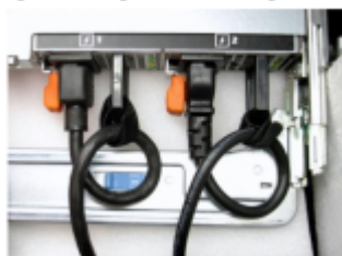
Figure 2: Routing Power Cables through the Strain Reliefs
