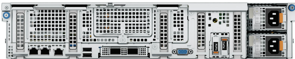
Figure 5. 5 x PCIe Low-Profile Slots
