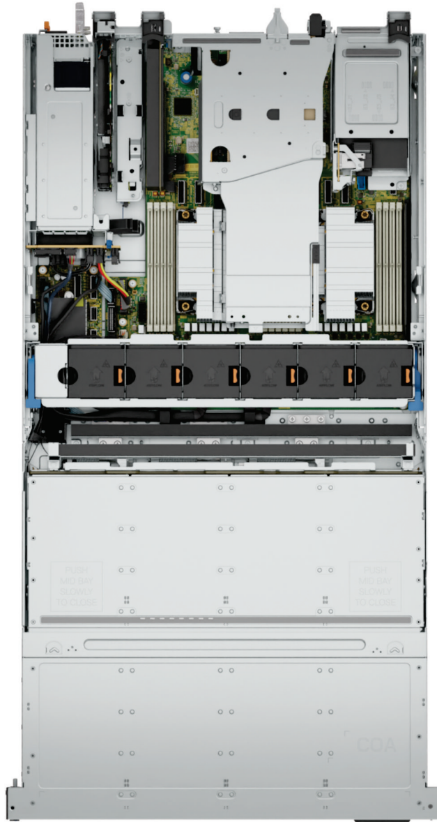
Figure 22. 2 x PCIe Low-Profile Slots + 2 x PCIe x16 FH/FL Slots + 4 x E3.S NVMe Drives
